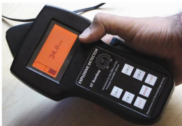
Figure 2. A low-cost hand-held device for the identification of explosives at airports, developed at IIT Mumbai.
