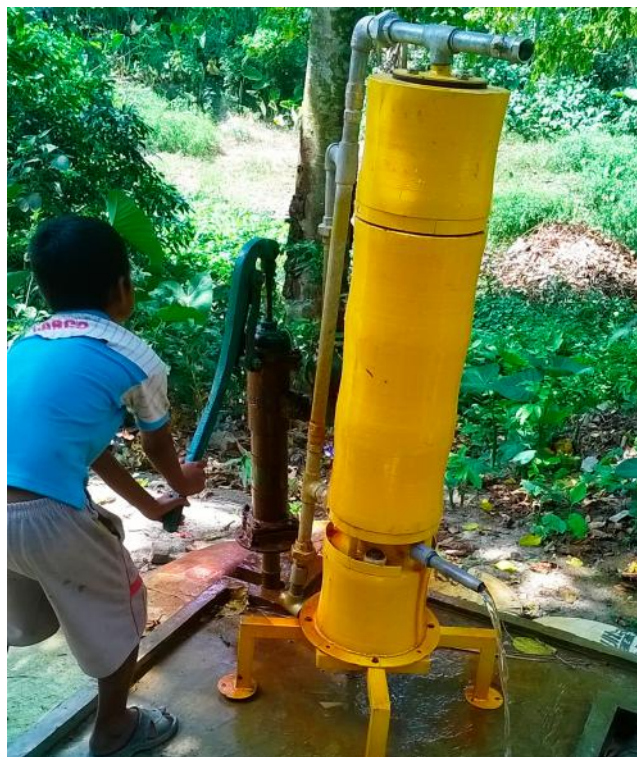
Figure 1. An arsenic and iron free drinking water product, named AMRIT, implemented by InnoNano Research Pvt. Ltd., in an arsenic-affected area of West Bengal, India. There are various versions of this technology, the one shown above caters to about 100 people. Arsenite and arsenate ions are removed well below the international norms at enhanced kinetic rates with sustainable granular materials. Such materials enable the design of a filtration column with a low pressure drop so that even a child can operate the filter. From the author's collection.
