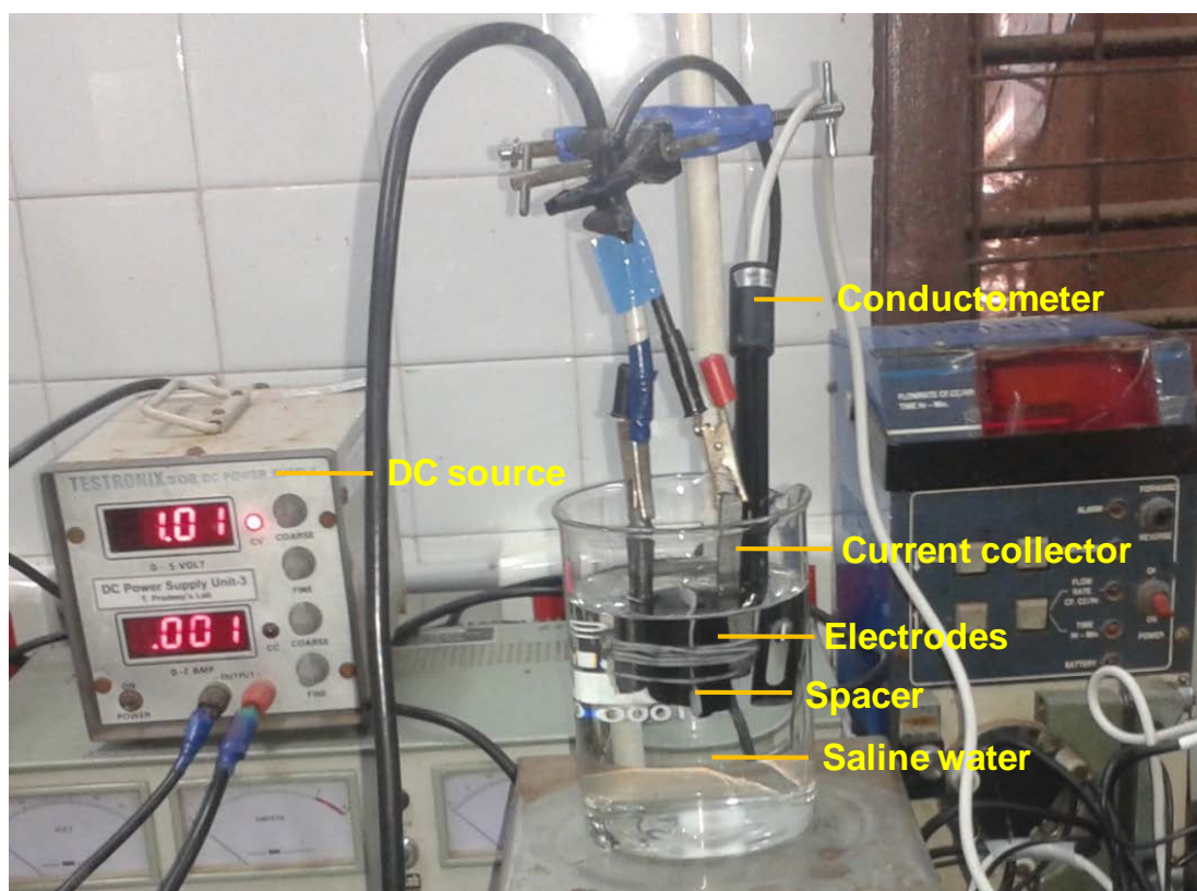
Fig. S7: Photograph of the CDI laboratory batch experimental set-up.
