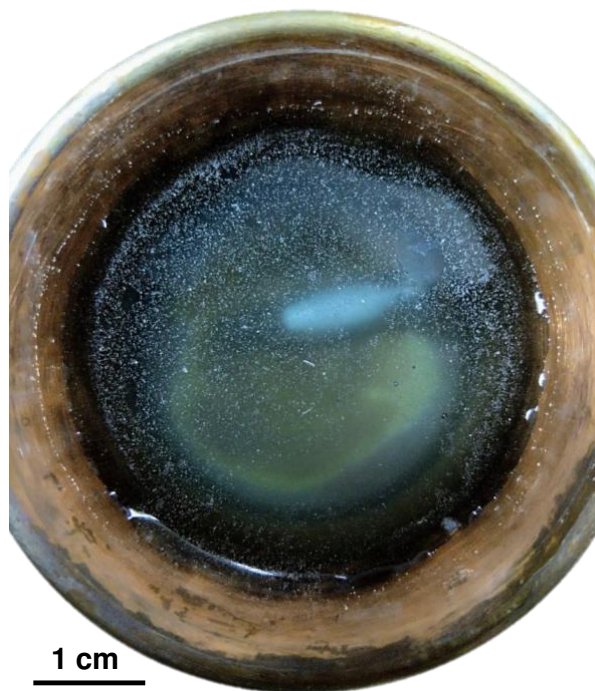
Figure S18. A) i) Photograph of the polypropylene vial. ii) A magnetic pellet was inserted into this vial. B) Reaction of polypropylene with glucose solution in copper vessel which was stirred to cause degradation. Degradation of polypropylene was noticed after 10 days of reaction. Spectroscopic and elemental analysis of the floating materials are presented in Figure S19–S20 and Figure S21, respectively.
