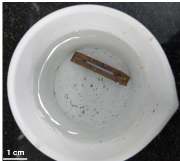
Figure S11. Reaction of PTFE pellet with copper chloride. Reaction of copper chloride solution (20 mg \text{CuCl}_2 in 50 mL water) with PTFE magnetic pellet in copper vessel A) and PTFE beaker B). Similar kind of degradation has been observed for copper (II) ions. Greenish blue color PTFE-metal composite has been observed. This reaction was performed without glucose.
