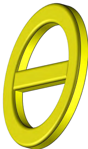
Figure S1. Schematic image of laser cut mesh from brass foil that is used for interfacial thickness experiment.
