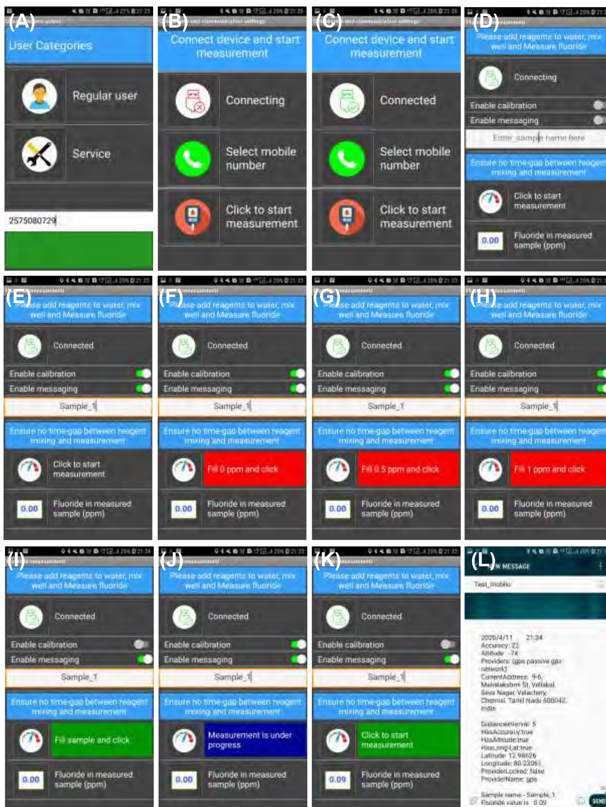
Figure S10. (A) to (L) show steps for using the fluoride sensor app over an android supporting phone for connection, calibration and measurements (output values not to be considered).
