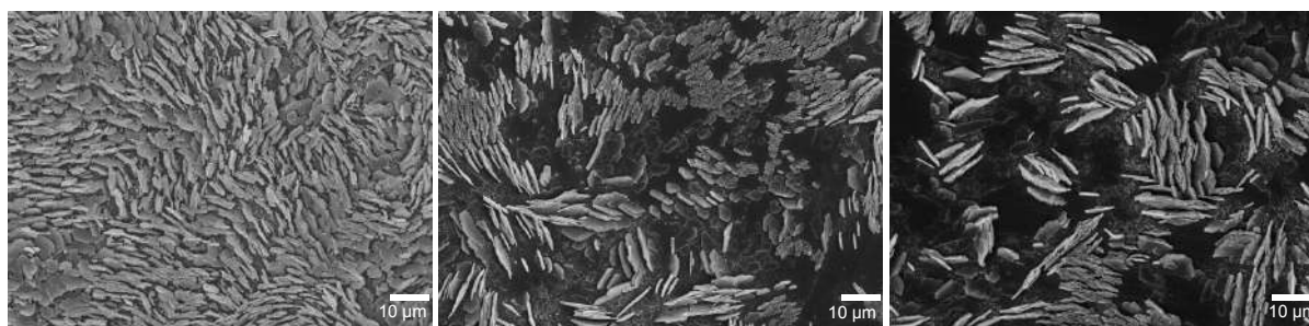
Figure S16. FESEM micrographs of three different films demonstrating reproducible nature of such nanostructures.
