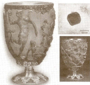
Figure 2: The Lycurgus Cup made from glass appears red in transmitted light and green in reflected light. The glass contains 70 nm particles as seen in an electron microscopic image. The cup itself is dated to 4th century AD, but the metallic holder is a later addition. 'Nano: The Essentials,' McGraw-Hill, 2008 10. T. Pradeep.
